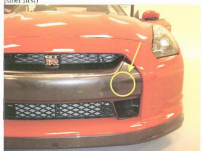
No hooks should be used to tie down vehicle to flatbed. Use of web straps is recommended (to prevent damage).
