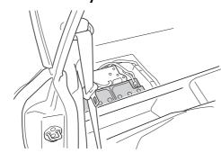
THE BATTERY IS LOCATED UNDER THE REAR STOWAGE FLOOR PANEL
