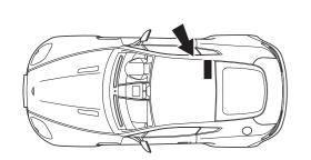
THE BATTERY AND BATTERY CONNECT SWITCH (BCS) ARE LOCATED BEHIND THE RH SEAT
